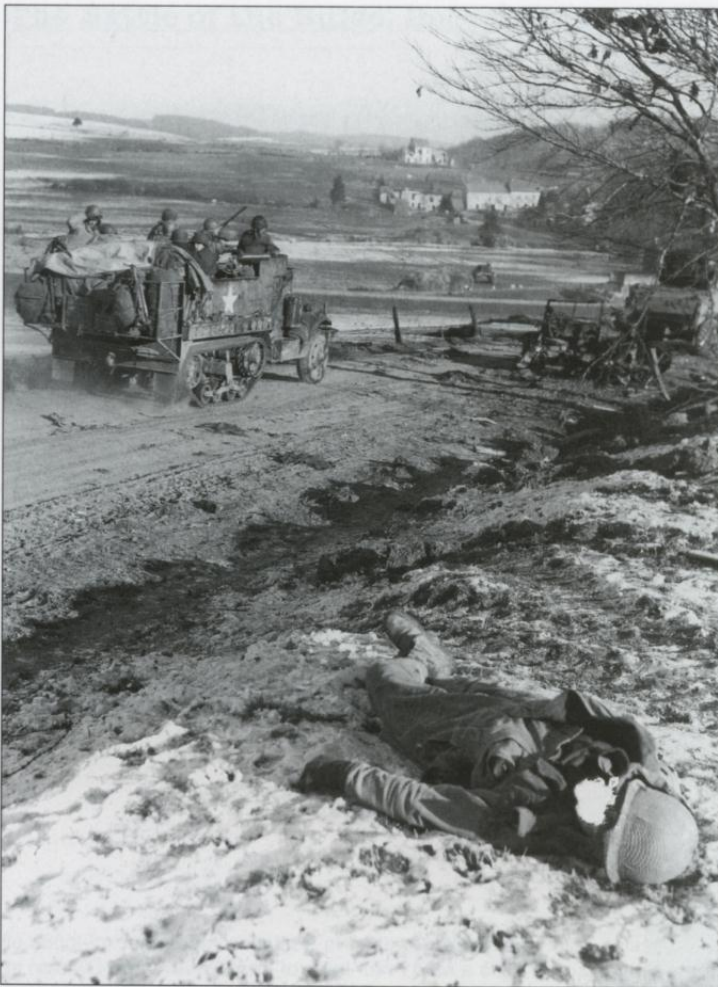
A M3A1 half-track from the 4th Armored Division moves forward through Chaumont in Luxembourg during the attacks to relieve Bastogne on 27 December 1944. The new folding rear stowage racks have been modified to permit stowage across the whole rear of the vehicle.
