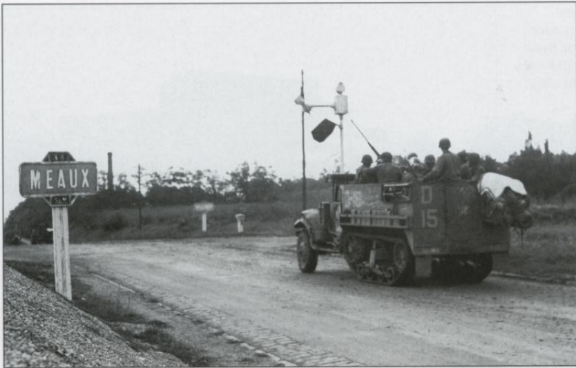
Another M3A1 half-track of the 3rd Armored Division, this time near Meaux, France on 28 August 1944. This division commonly marked its vehicles with the company letter as well as with its radio call number. The large bright colored cloth panel on the corner of the vehicle is a fluorescent pink or yellow air identification panel.
