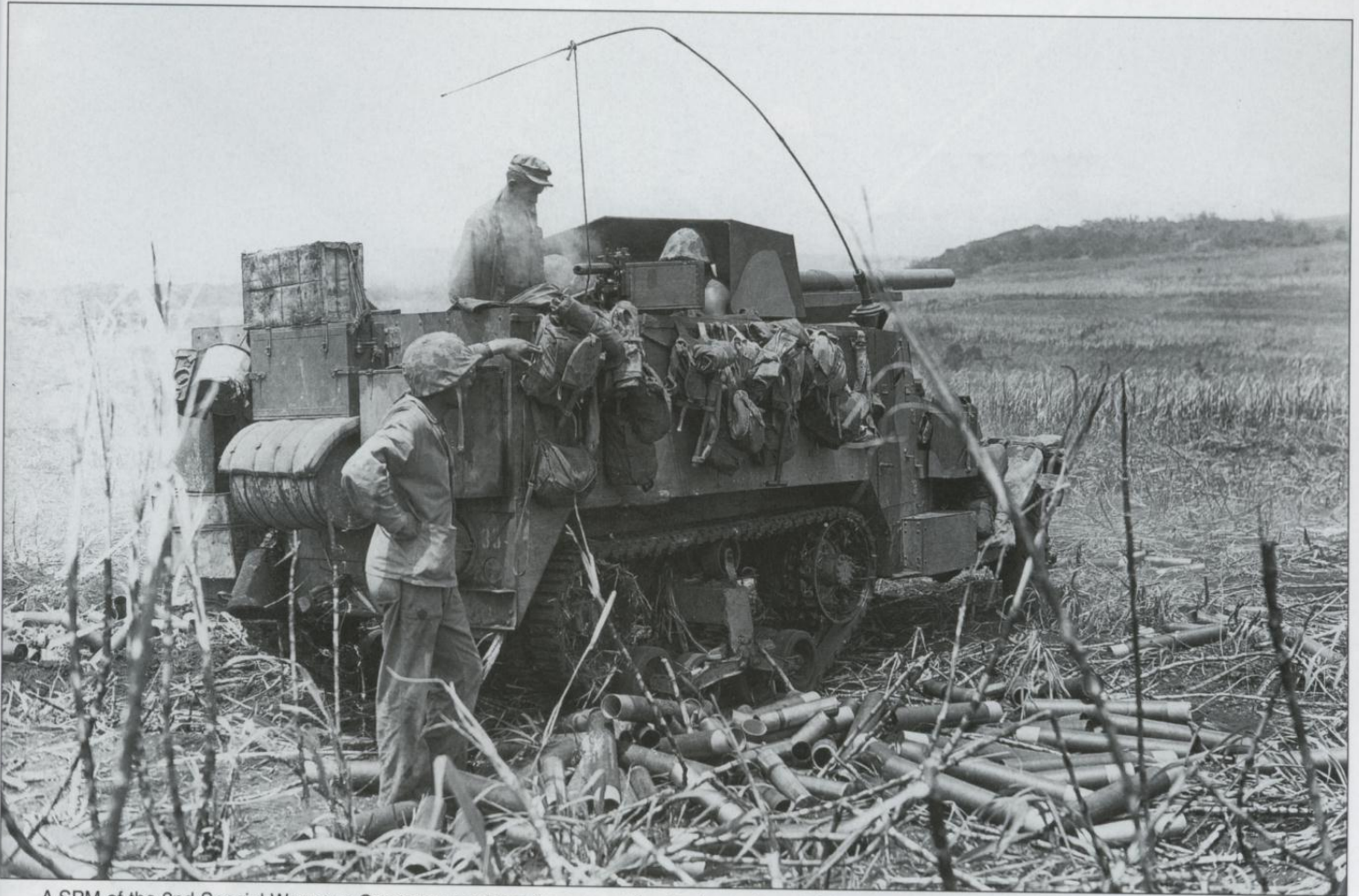
A SPM of the 2nd Special Weapons Company providing fire support for Marine units on Tinian on 30 July 1944. The ground near the vehicle is littered with packing tubes and expended brass shell casings. These vehicles were used on occasion in their intended role as tank destroyers, including engagements on Peleliu and Saipan.
