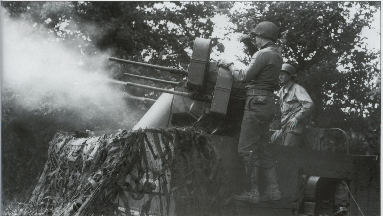
A multiple gun motor carriage of the 377th AAA Battalion is being used to provide fire support for an infantry unit in Normandy on 12 July 1944. There was so little German air activity over the beachhead that many anti-aircraft units were sent forward to provide fire support. This is some sort of expedient M16 as careful inspection reveals it is mounted on a M2 half-track chassis, not the normal M3, and does not have the characteristic folding sides.
