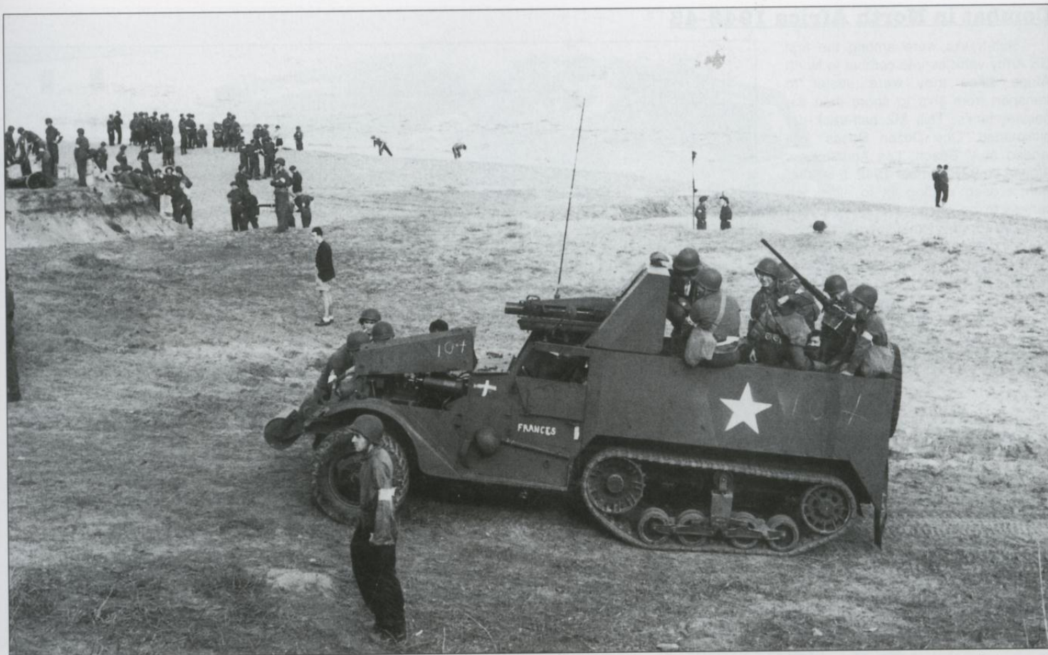
A T30 75mm HMC shortly after having landed near Algiers on 8 November 1942. These landings were conducted mainly by infantry units, but a small number of T30 75mm HMC and T19 105mm HMC were landed to provide fire support.
