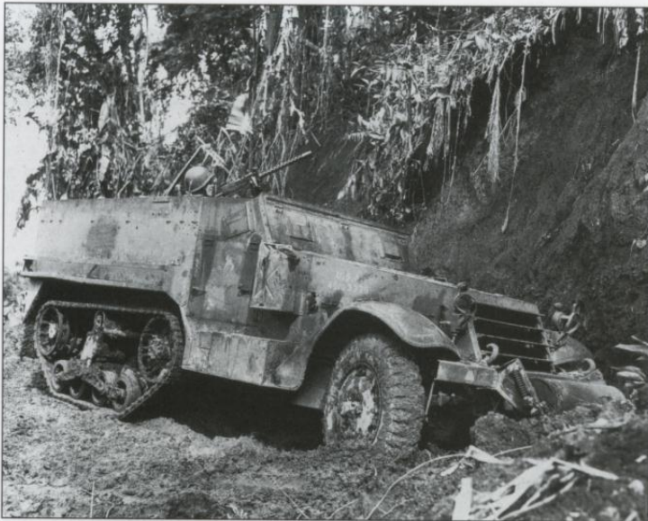
The US Army did not use armored infantry battalions in the Pacific but did use half-tracks in reconnaissance, headquarters and communications units. This is a M3 half-track of the 37th Recon Troop used during the fighting on Bougainville on 10 March 1944.
