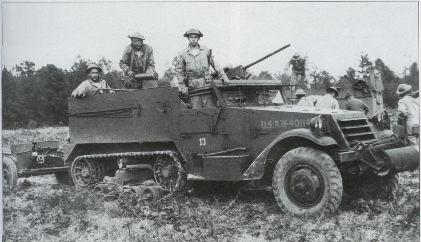
The M2 half-track car was commonly used for towing infantry support weapons such as this M3 37mm anti-tank gun with the 6th Infantry Anti-Tank Company, in Jefferson, North Carolina, in November 1941. The cloth band on the hull side is a colored marker used to distinguish opposing forces during war-games.
