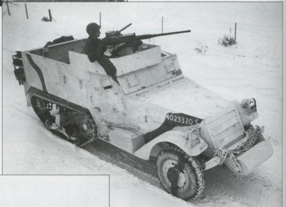
The XX Corps encouraged the pattern painting of armored equipment using whitewash, and this particular M2A1 half-track car was displayed as an example. The dark bands are from the original olive drab finish.
