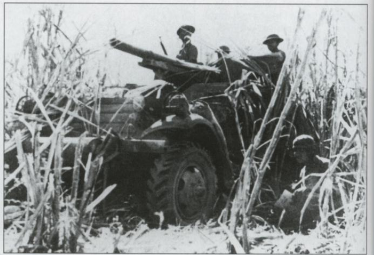
The first combat use of half-tracks came in December 1941 in the Philippines. The Provisional Tank Group was equipped with 46 M2 and M3 half-tracks, as well as 50 T12 75mm gun motor carriages. The T12 was intended as a tank destroyer and mounted the American version of the legendary French "soixante-quinze" canon of World War I fame. When standardized, it was designated as the 75mm M3 gun motor carriage (GMC). (Michael Green)
