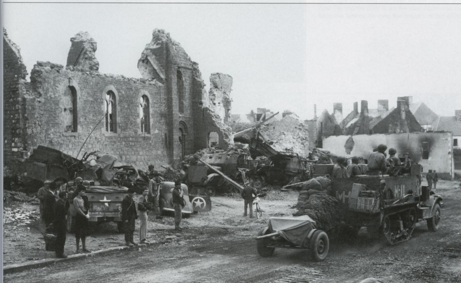
A M3A1 half-track of the 3rd Armored Division passes through the ruins of Roncey on 1 August 1944. In the wreckage is a destroyed Sd.Kfz. 7 fitted with a quadruple 20mm anti-aircraft gun and a 7.5cm Pz.Jäger 38(t) Ausf. M (Sd.Kfz. 138) tank destroyer of the SS-Pz.Jg.Abt.2 of the 2.SS-Panzer-Division. The M3A1 half-track is towing a 37mm anti-tank gun, a weapon inadequate for anti-tank defense in 1944.
