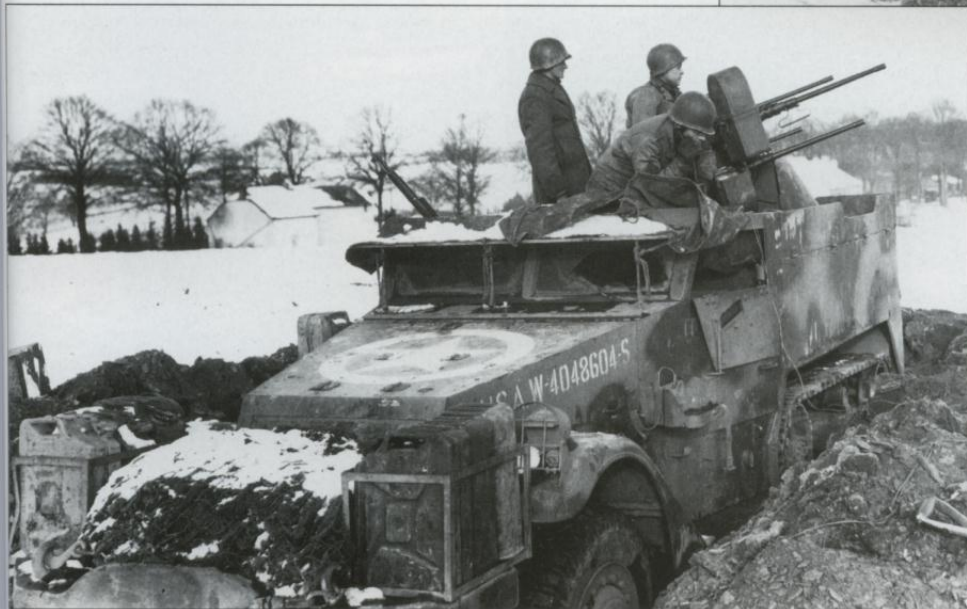
A M16 MGMC of the 447th AAA Battalion is dug in near Neufchateau, Belgium on New Year's Day, 1945. The vehicle has jerry can racks added on the winch bumper and is pattern painted with black camouflage paint over the usual olive drab.
