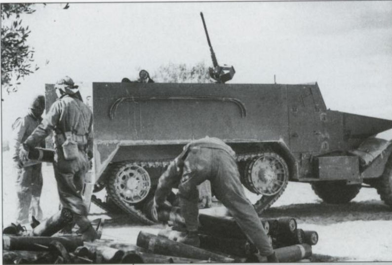
A close-up of a M3 half-track used as an ammunition carrier during fighting near Sbeitla on 17 February 1943. The devices on the hull side are hoops for a canvas cover that could be placed over the open troop compartment.
