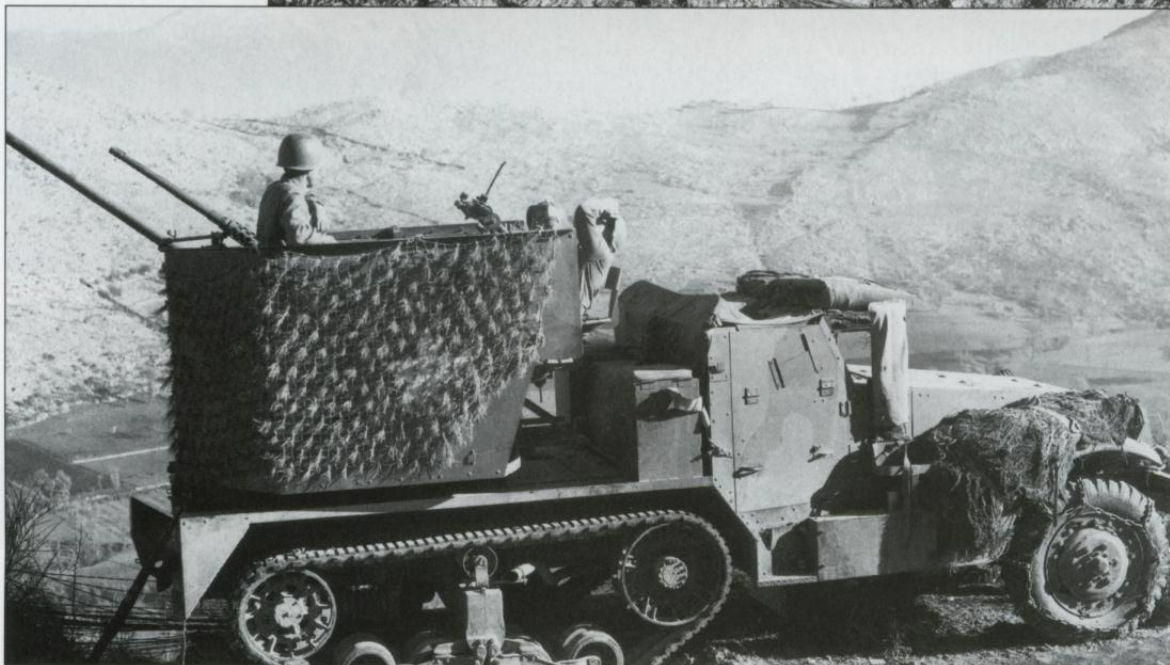
A M15 of Battery D, 105th AAA battalion near San Pietro on 8 January 1944. A camouflage net is fitted to the rear turret, and the vehicle also has pattern painted camouflage, probably black over olive drab.
