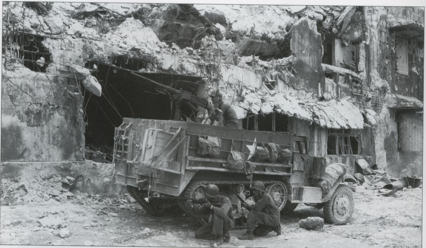
A M3 half-track in action near a wrecked plant on Peleliu island, Palau in the Caroline Islands in 1944. Curiously enough, the exhaust extension is vented up through the cab rather than outside the cab as on most deep wading kits.
