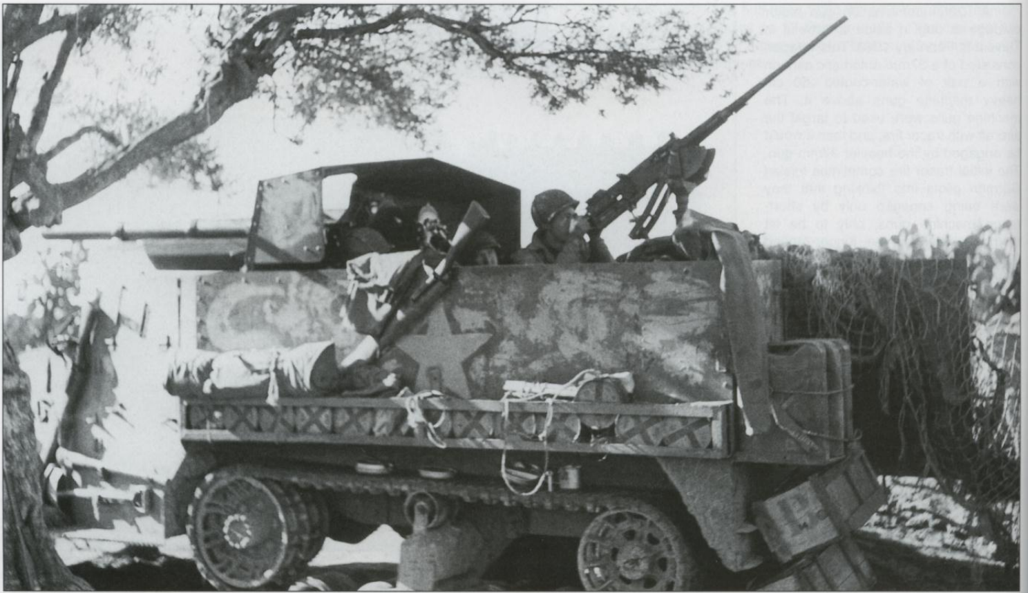
A M3 75mm gun motor carriage uses the camouflage provided by a tree during fighting in Tunisia in the spring of 1943. The improvised mud camouflage used in Tunisia is very evident in this view. The threat of air attack was constant in Tunisia, and pintle mounted heavy machine guns were a common feature.
