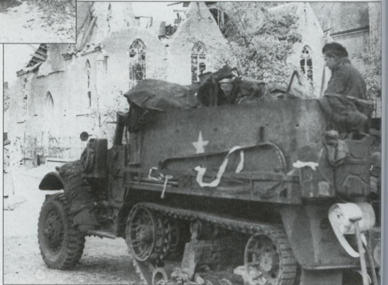
Another view of an M5A1 or M9A1 of the 11th Sapper Company, 1st Polish Armoured Division in France in August 1944 during the assault towards Falaise. This vehicle has rolls of white tape that were used to mark cleared lanes through minefields. (Sikorski Institute)
