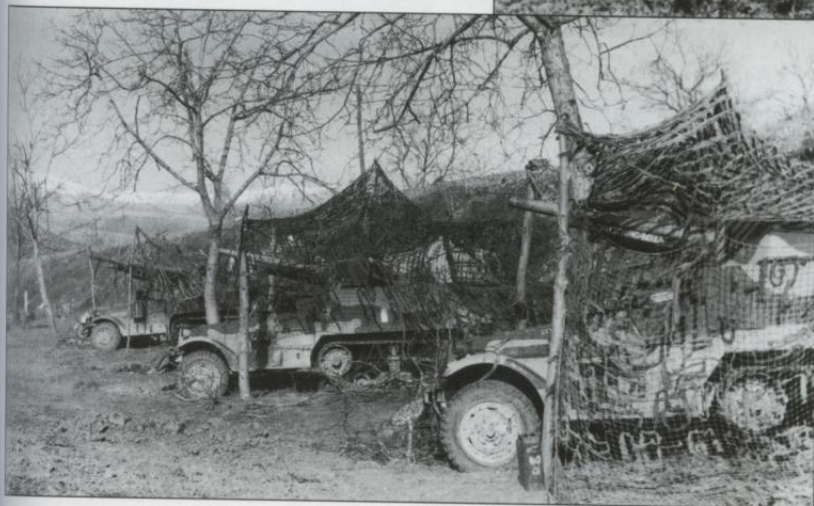
Already by 10 April 1944 when this photo was taken, the newer M16 multiple gun motor carriage was available and was first deployed in combat in the Anzio beachhead. This vehicle had four .50 cal heavy machine guns instead of two, but was otherwise similar to the M13 MGMC.
