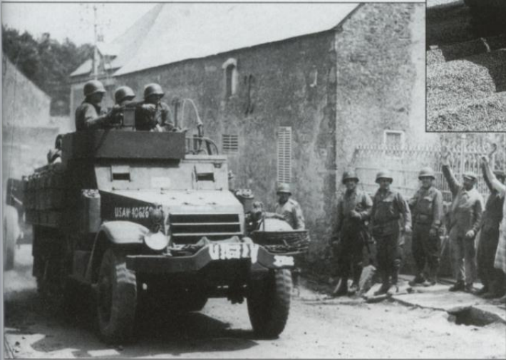
A M3A1 half-track moves through a French village in Normandy on 13 June 1944. The Army censor has painted out the unit codes on the winch bumper. This vehicle is towing one of the new M6 76mm anti-tank guns, and so is presumably from an anti-tank company of an armored division.
