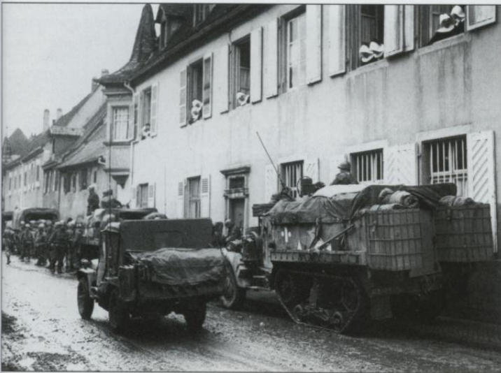
A M3A1 half-track of the 119th Engineers, 12th Armored Division rest in the town of Rouffech, France on 5 February after the Colmar pocket had been sealed. The vehicle is fitted with a locally built stowage rack on the rear. This half-track is marked with the "bar and ball" geometric tactical insignia peculiar to the 12th Armored Division.
