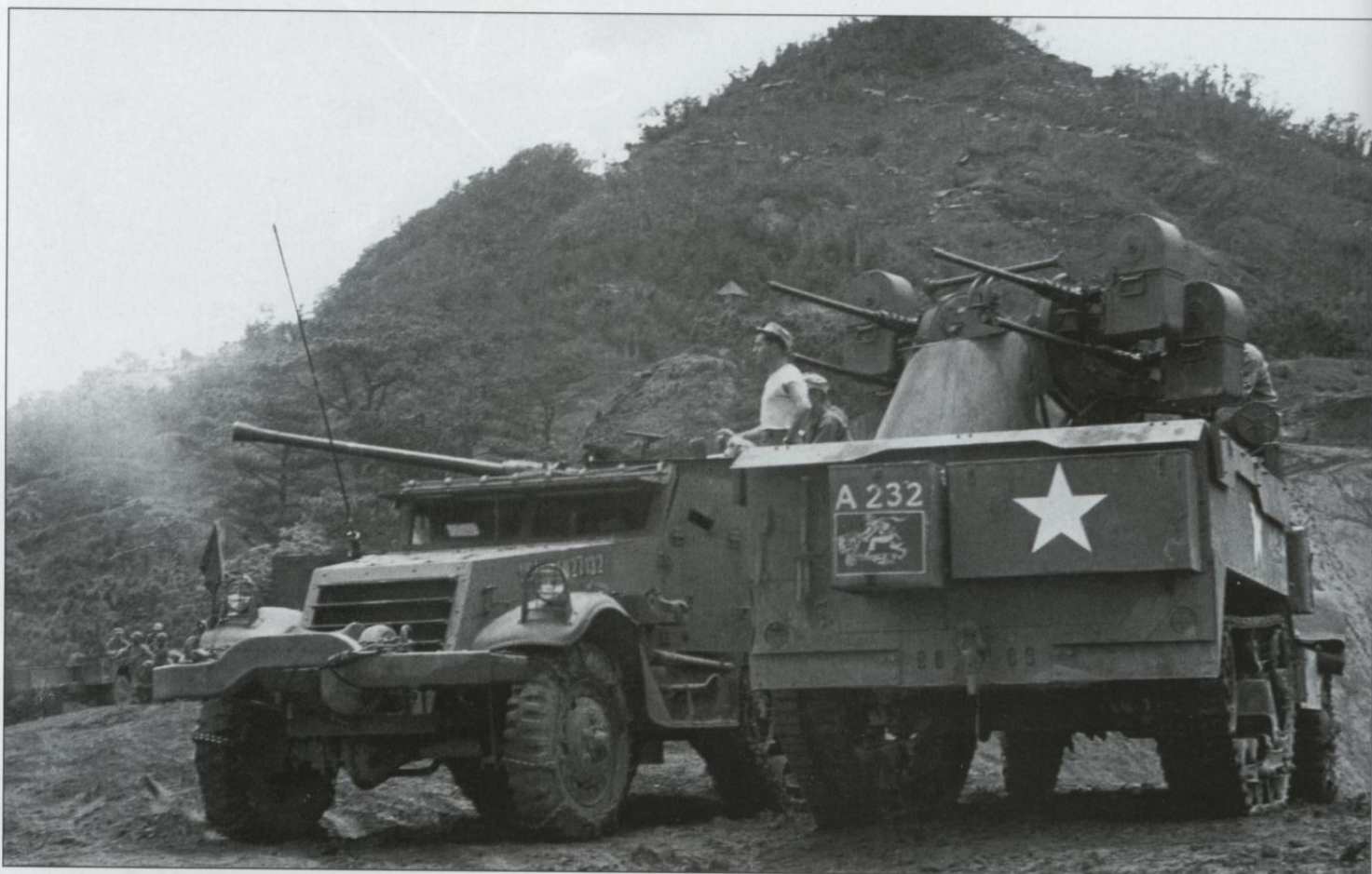
An interesting shot showing both a M15 Special and a M16 MGMC of the 209th AAA Battalion providing fire support for the 32nd Infantry Division near Yamashita Ridge on the Villa Verde Trail in the Philippines on 17 August 1945. The elaborate cartoon insignia is repeated on the side of the M16 as well.
