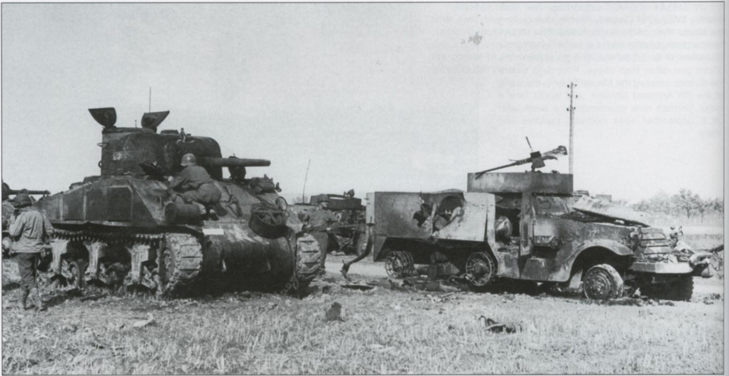
US troops inspect a knocked out column of armor outside Nancy, France on 10 September 1944 during the initial stages of the fighting for Lorraine. These are probably from the 4th Armored Division. The M3A1 half-track has been hit by a high explosive round which has caved in the side armor and set the vehicle on fire.
