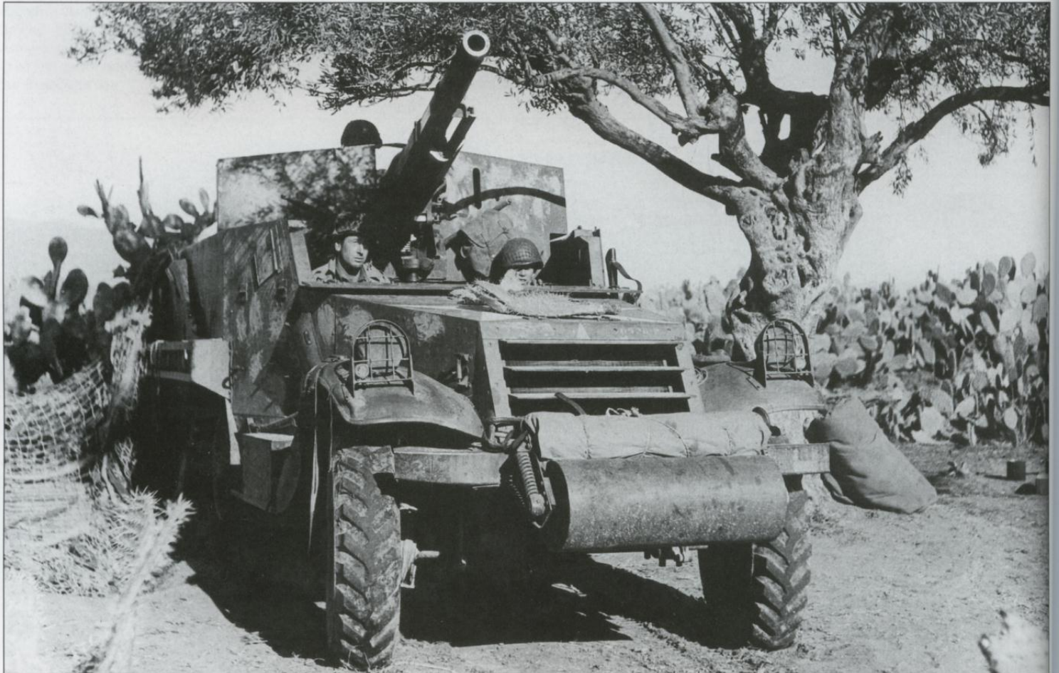
A view of the front of the same tank destroyer. This vehicle is fitted with the initial pattern headlights. These were replaced with a type of detachable headlight, since the fixed headlights were often destroyed or damaged from the muzzle blast of the gun firing.
