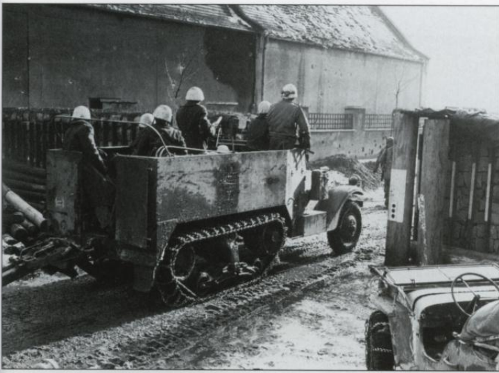
With the Ardennes bulge eliminated, the Allied armies began pressing ahead towards Germany. Here a M3 half-track of the French 2nd Armored Division passes through a tank barrier in the outskirts of Colmar on 2 February 1945. The rear tracks have a set of chains added for better traction in the snow.
