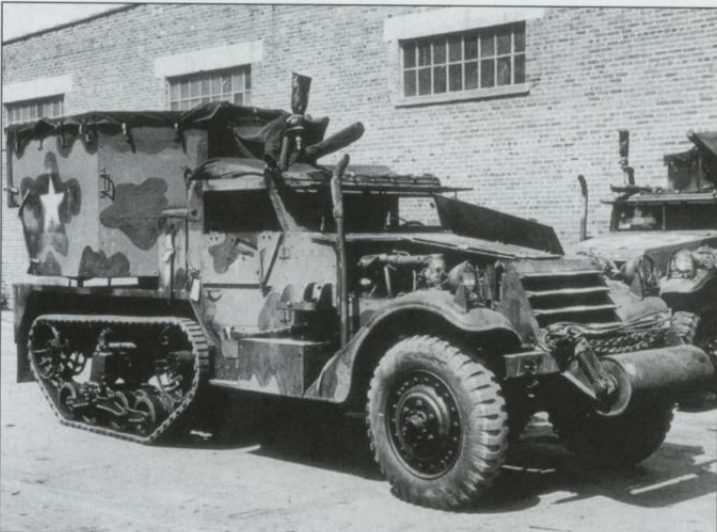
An M15 combination gun motor carriage is prepared for shipment to the Mediterranean theater in 1943 at an Atlantic coast port. The M15 was an upgrade of the T28E1, most easily distinguished by the use of an armored basket around the gun mount. This vehicle is painted in a disruptive scheme of black over olive drab.
