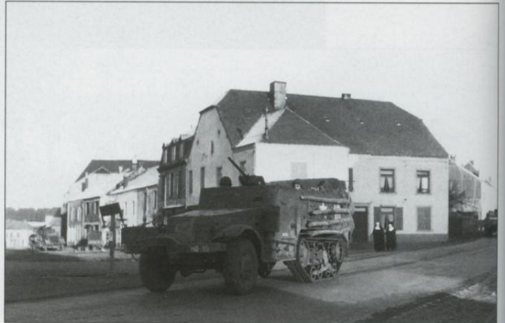
An older M3 half-track named "Helen" of a headquarters unit from the 6th Armored Division moves through Habay-la-Neuve, Belgium during the Ardennes fighting on 29 December 1944. The chain of logs lashed to the side were used to help unditch the vehicle's forward wheels if soft mud was encountered.
