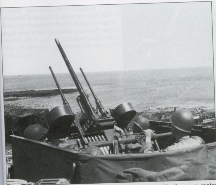
A detailed view of the gun tub of a M15A1 combination gun motor carriage. The twin .50 cal machine guns were usually used to bring the target under fire and range it, after which the more powerful 37mm automatic cannon was engaged.
