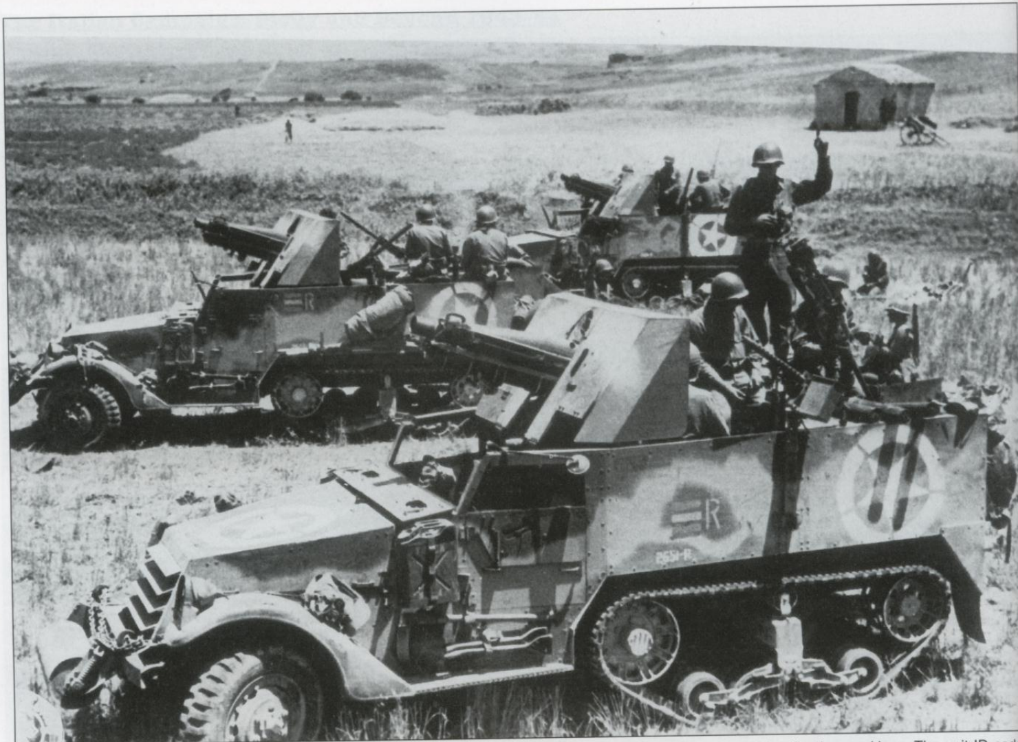
A close-up of the T30 howitzer motor carriages at Licata. The three color bars on the vehicle side are unit identification markings. The unit ID code, 2651-R can be seen below the bars. From the last two digits of the unit code, the bars colors were light gray top and bottom and blue in the center. The vehicle is finished in the usual ANA 305 earth yellow over olive drab, the official pattern ordered for Husky.
