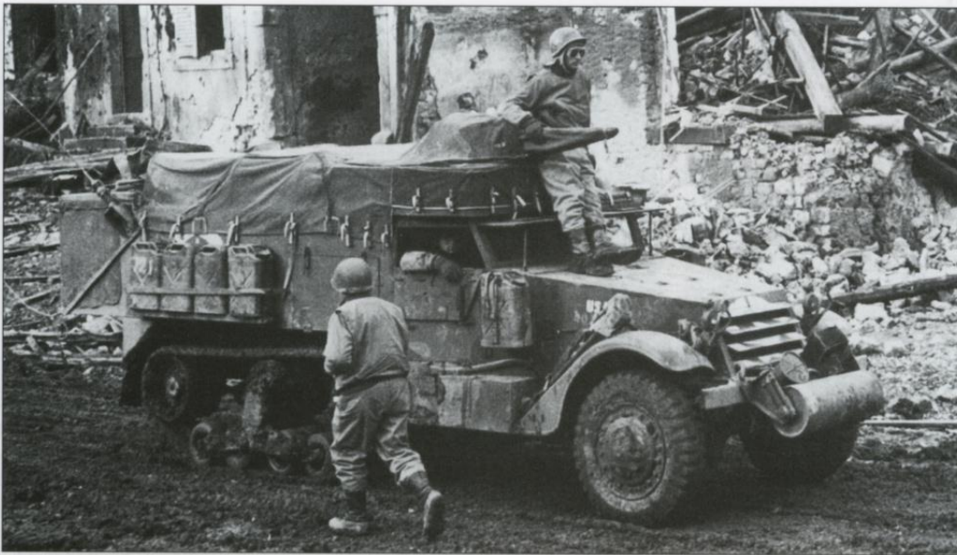
A M2A1 half-track car passes through the ruins of Xosse, France on 18 November 1944. The side mine rack has been converted to carry jerry cans of fuel or water.
