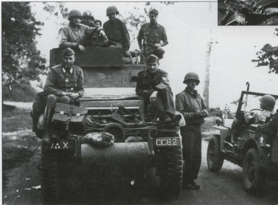
A M3A1 half-track of the Combat Command B headquarters from 7th Armored Division, named "Lucille-B". The extra radio antennas typical of a headquarters vehicle are evident here. There is an air identification panel adjacent to the machine gun pulpit. (Withers collection, Patton Museum)
