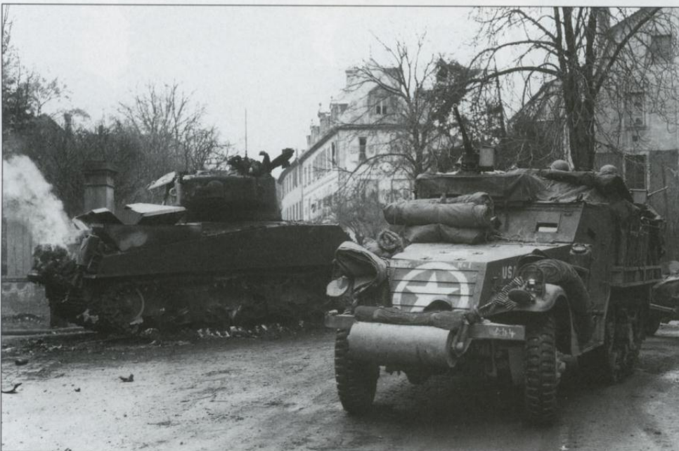
A M3A1 half-track named "Baby Bastard No. 1" passes the burning wreck of a M4A3 (76) medium tank of the 48th Tank Battalion, 14th Armored Division, knocked out during the fighting in Barre, France on 29 November 1944.
