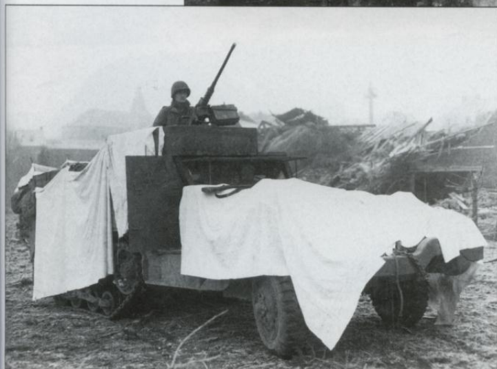
Lacking paint, some units trapped in Bastogne tried other methods of snow camouflage. This is a M3A1 half-track of the 10th Armored Division in Bastogne on 27 December 1944 using white sheets.
