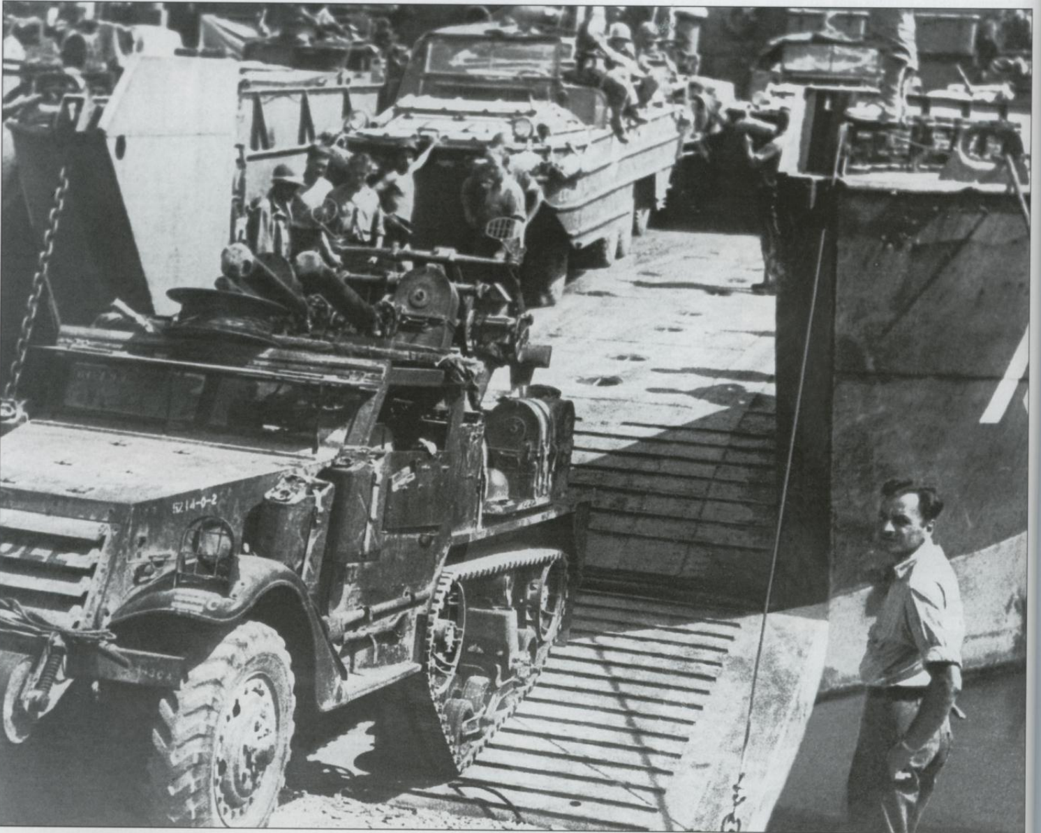
A T28E1 combination gun motor carriage of the 3rd Infantry Division is loaded into an LCI alongside some DUKWs in preparation for Operation Husky: the invasion of Sicily. The vehicle carries the unit bar codes of 5214, and so the three colored bars evident below the headlight are blue/yellow/blue.
