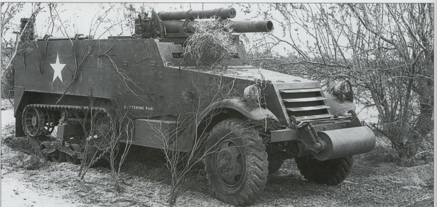
"Battering Ram", a 105mm T19 HMC during training at the Desert Training Center in the Mojave desert in southern California on 26 January 1943. The initial production batches of the T19 HMC lacked a gun shield for the crew.
