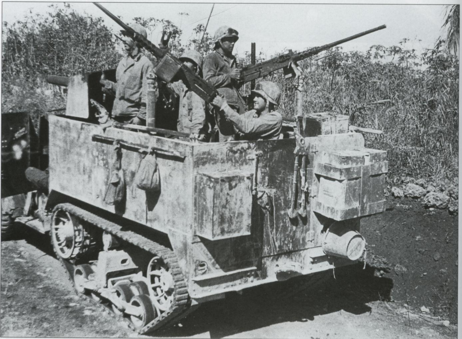
A well armed Marine SPM of the 4th Special Weapons Company on Saipan in June 1944 with two heavy pintle mounted .50 cal heavy machine guns on either side, two smaller pintles for .30 cal machine guns forward of these, and a third .30 cal pintle over the gun shield. The profusion of machine guns was due to the fact that these vehicles were often called upon to engage Japanese infantry where automatic weapons fire was more effective than the gun. (USMC)
