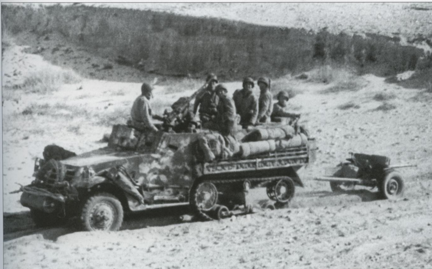
A M3 half-track of the 1st Armored Regt., 1st Armored Div. near Sidi-bou-Zid on 14 February 1943, towing a M3 37mm anti-tank gun. By this stage of the fighting, US forces had begun to use an improvised mud camouflage on their olive drab vehicles to help them better blend in to the desert background.
