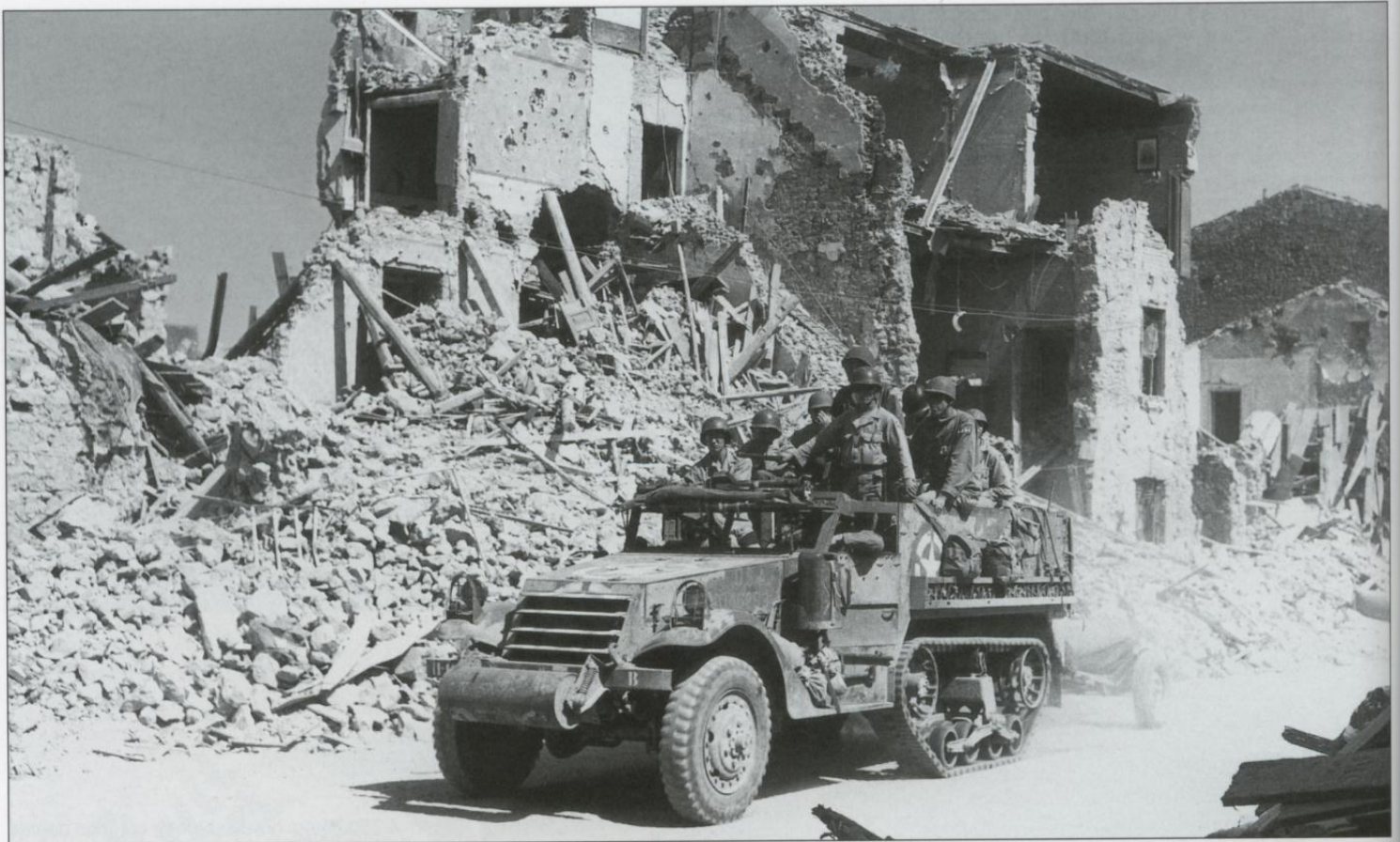
A M3 half-track towing an M3 37mm anti-tank gun passes through the ruins of a Sicilian village. This particular vehicle was attached to a headquarters unit of Bradley's 2nd Corps, and the troops in the vehicle are wearing the 2nd Corps patch.
