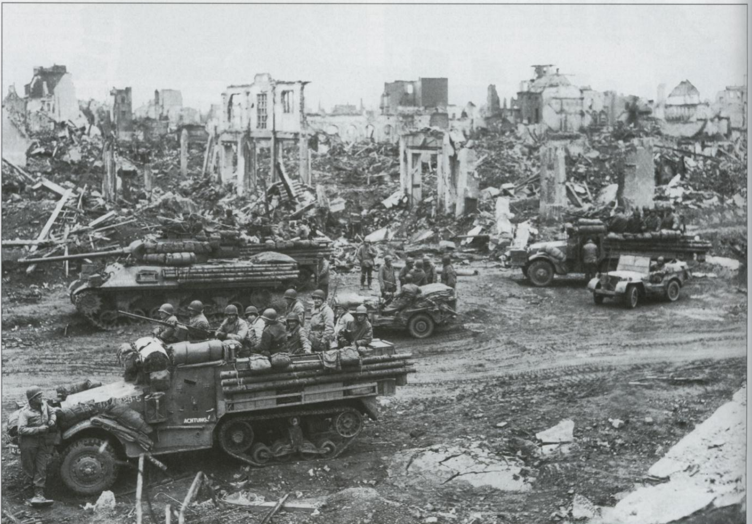
In the foreground is a M3A1 half-track named "Achtung!" of the 23rd Engineers, 3rd Armored Division while in the background are other vehicles from the unit including a M36 90mm tank destroyer. The unit is passing through the ruins of Dueren, Germany on 26 February 1945. Dueren had been hotly contested due to its strategic position on the Roer river, and it was a staging area for the VII Corps' Roer river crossing during Operation Grenade in late February 1945.
