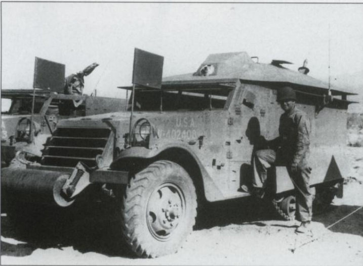
Besides authorized variants, US troops were prone to develop their own derivatives of the half-tracks. This is a M3 half-track rebuilt as a command vehicle on the instructions of Lt. Gen. George S. Patton during his stint at the Desert Training Center. Patton loved to tinker with customized vehicles, and while in command of the 1st Armored Corps in Tunisia, used a customized M3A1 Scout Car.
